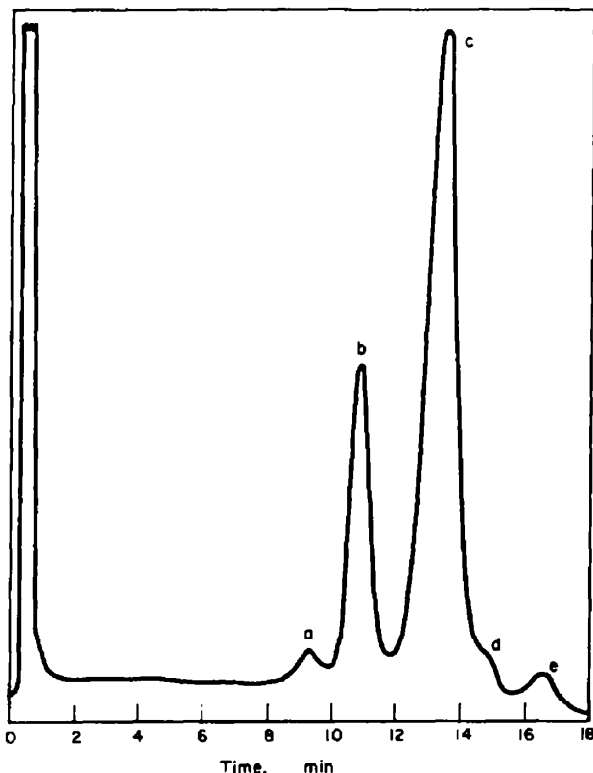
FIG. 4. Gas chromatography of methyl ester fraction, b.p. 240–247°/2 mm, from a combined lot of lipids from tubercle bacillus (fifth item, Table 3). Chromatography on column described for Fig. 1; temp 267°; helium flow rate, 70 ml/min; initial off-scale band from solvent. Material collected from the lettered bands is described in Table 1 (except for Band e , assigned to methyl C 30 -phthianoate), and semi-log plots of the retention times are included in Fig. 5.
